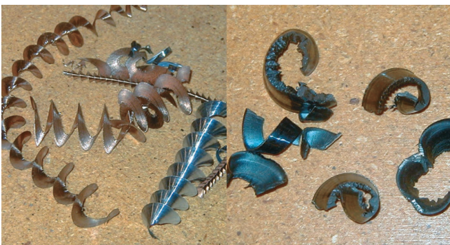
Figure 1-19 Long, stringy chips are strong razor wires that catch clothing and cut skin. All chips, even the safer “C” shapes on the right, can be dangerously hot. ©McGraw-Hill Education/Lake Washington Technical College, Kirkland, WA
