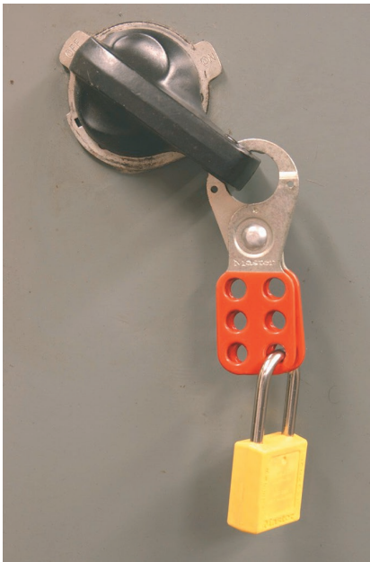
Figure 1-21 Lock it out or lock it up—never perform maintenance on a machine that can be started accidentally. ©McGraw-Hill Education/Photography by Prographics at Milwaukee Area Technical College
