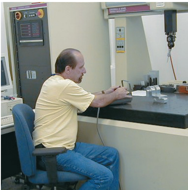
Figure 2-2 This machining inspector needs math skills to read the drawing and then program this computer coordinate-measuring machine (CMM). Courtesy Contour Aerospace/Everett, WA
