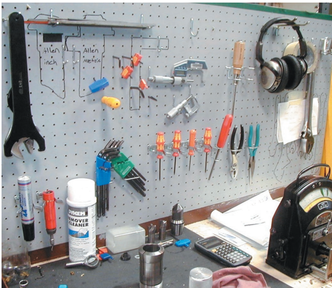
Figure 1-29 A lean shadow board and machine. Courtesy Tye Aircraft, Everett, WA
