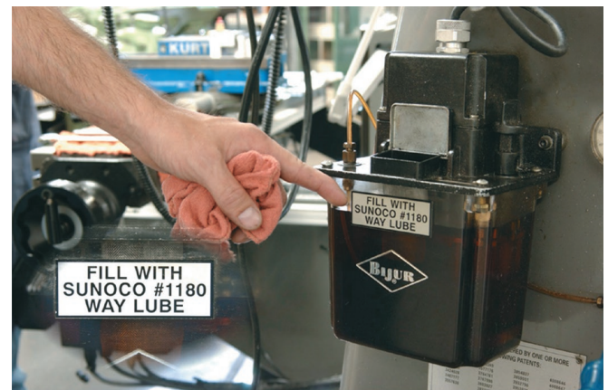
Figure 1-16 Be absolutely certain to add the right oil, especially on CNC equipment! ©McGraw-Hill Education/Lake Washington Technical College, Kirkland, WA
