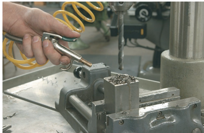
Figure 1-25 Compressed air is a good chip removal and cleanup tool when correctly used. ©McGraw-Hill Education/Lake Washington Technical College, Kirkland, WA
