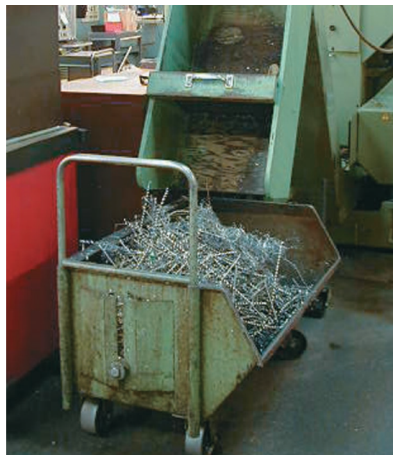
Figure 1-20 Chips can pile up quickly and must be removed from the machine. Courtesy Mike Fitzpatrick
