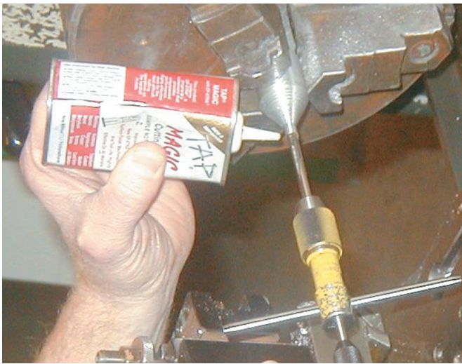
Figure 1-18 Thread-cutting compound makes a huge difference in thread quality and tool life, but it is expensive. ©McGraw-Hill Education/Lake Washington Technical College, Kirkland, WA
