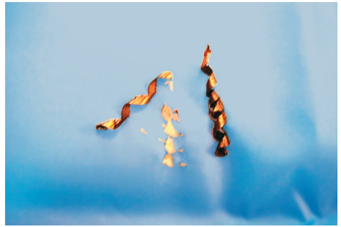
Figure 1-5 Two hot chips melted onto this nylon windbreaker while the center one went completely through to possibly burn the person within! Courtesy Mike Fitzpatrick
