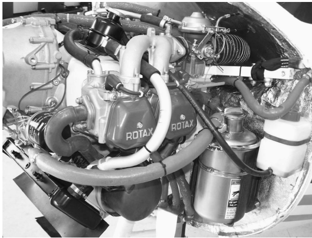
FIGURE 1-24 Typical four-cylinder, four-stroke horizontally opposed engine.
