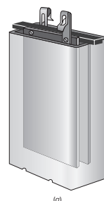
Figure 1-8 Chemical cell as a voltage source. (a) Voltage output is the potential difference between the two terminals. (b) Schematic symbol of any DC voltage source with constant polarity. Longer line indicates positive side.
