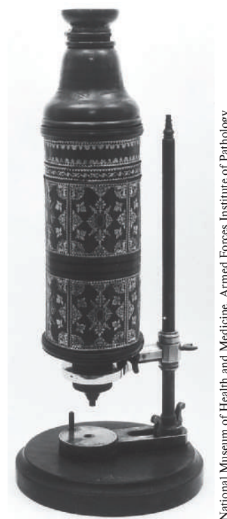
Figure 2.2 Robert Hooke's microscope.
