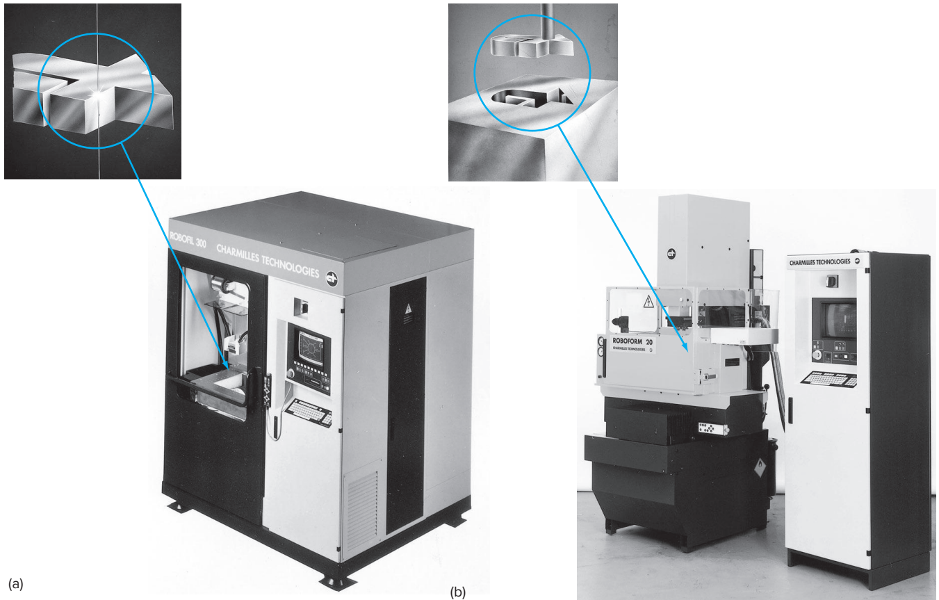
■ Figure 1-12 EDM machines remove metal by an electric spark-erosion process. (Courtesy of Charmilles Technology Corp.)
