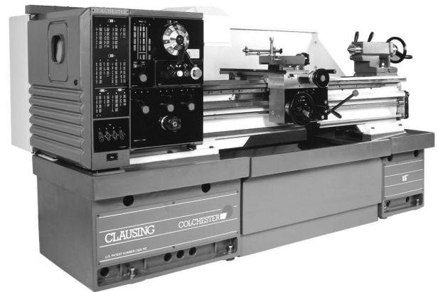
■ Figure 1-6 An engine lathe is used to produce round work. (Courtesy of Clausung Industrial, Inc.)
