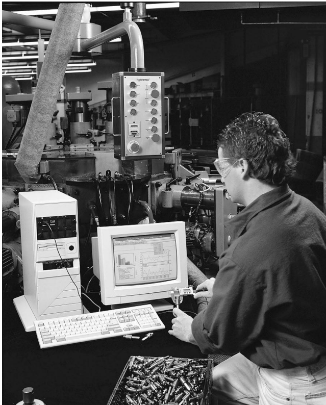
■ Figure 2-8 Inspectors check the dimensions of finished parts and products. (©Steve Krar)
