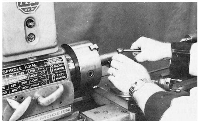
■ Figure 4-4 Wearing rings and watches can cause serious injury. (©Kelmar Associates)
