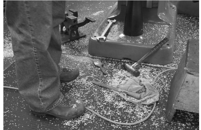
■ Figure 4-8 Poor housekeeping can lead to accidents. (©The McGraw-Hill Companies, Inc./Photographer Prographics, Inc.)
