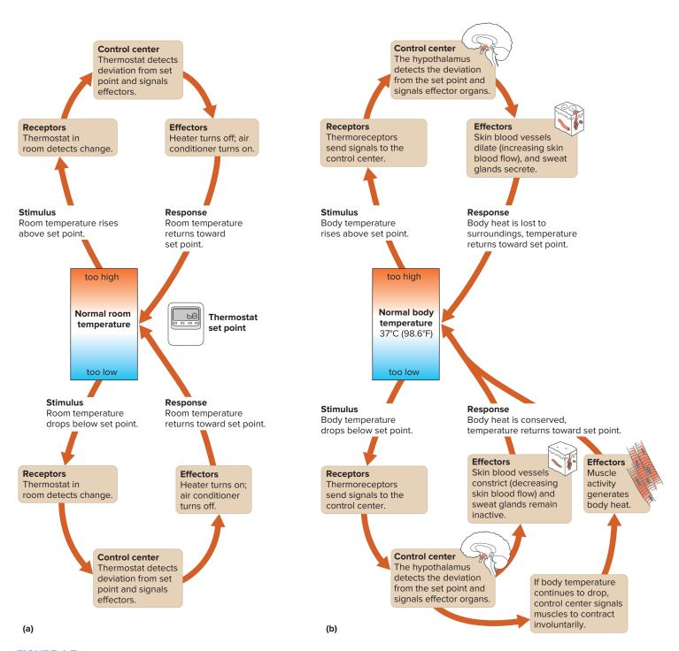
**FIGURE 1.7** Negative feedback. (a) A thermostat signals an air conditioner and a furnace to turn on or off to maintain a relatively stable room temperature. This system is an example of a negative feedback loop. (b) The homeostatic mechanism that regulates body temperature is a physiological example of a negative feedback loop.
