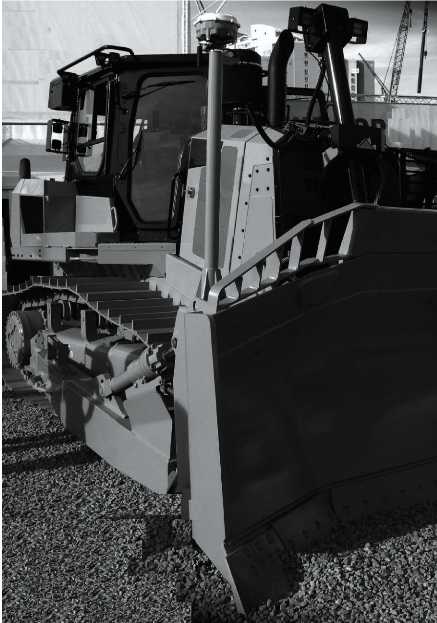
FIGURE 1.4 Automatic blade control mounted on a dozer
