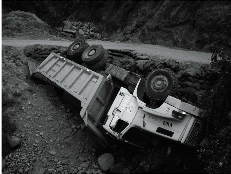
FIGURE 1.5 Loaded trucks can easily overturn
