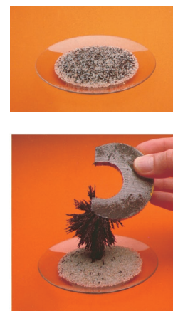
Figure 1.7 An example of separation based on differences in physical properties. Magnetic iron is separated from nonmagnetic substances. A large-scale version of this process is important in the recycling industry.
