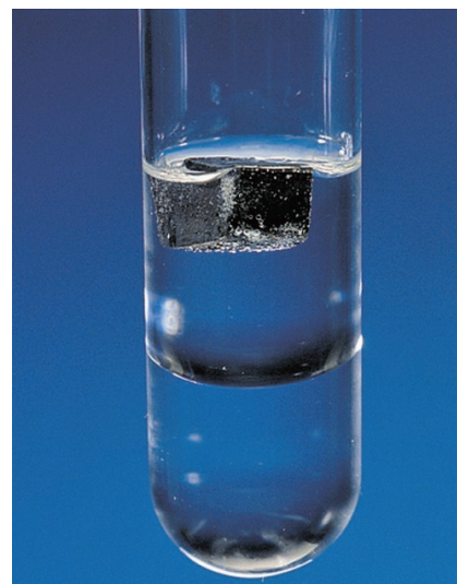
Figure 1.13 Density (mass/volume) is a unique property of a material. A mixture of water and oil is shown, with lithium—the least dense—floating on the oil. The oil, with a density greater than lithium, but less than water, floats on the interface between lithium and water. ©McGraw-Hill Education/Stephen Frisch, photographer
