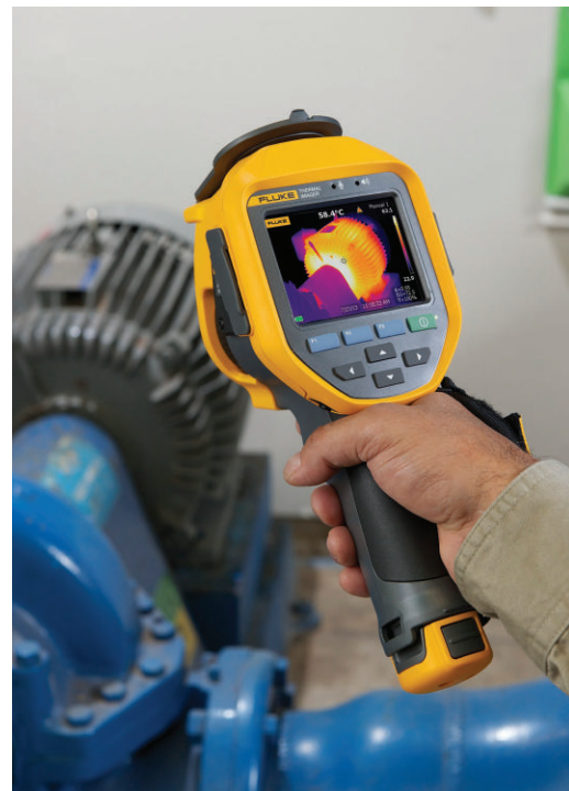
Figure 2-42 Motor thermal imaging inspection.
