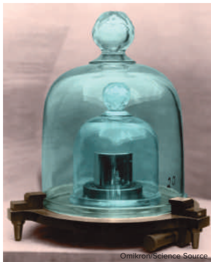
FIGURE 3.3 One of the kilogram standards kept at the U.S. National Bureau of Standards. This platinum-iridium cylinder is stored under vacuum to reduce chemical reactions that might change its mass.
