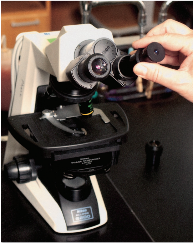
Figure 3.6 If the ocular of a phase-contrast microscope is replaced with a centering telescope, the orientation of the phase ring and annular ring can be viewed.
