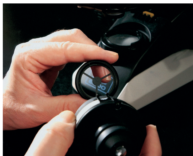
Figure 2.2 The insertion of a star diaphragm into the filter slot of the condenser will produce a dark field suitable for low magnifications.
