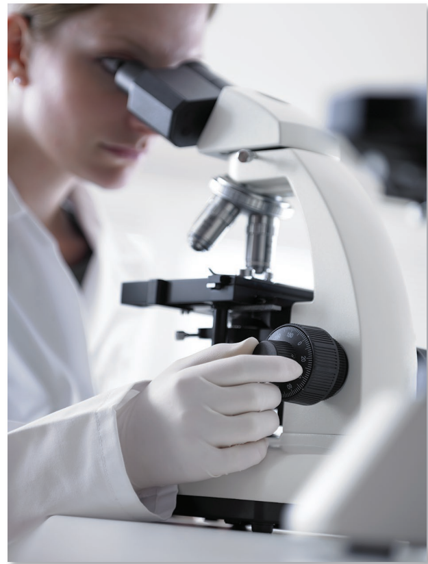
Figure 1.6 When you are using the high-dry or oil immersion lens, use only the fine adjustment knob.
