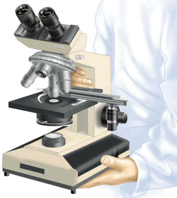
Figure 1.5 The microscope should be held firmly with both hands while being carried.
