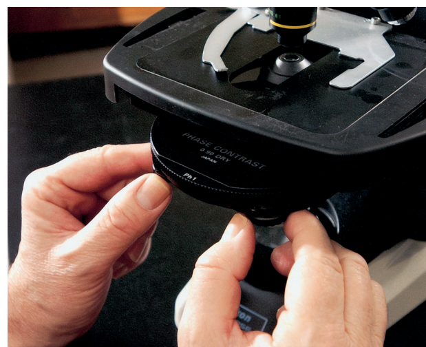
Figure 3.5 Alignment of the annulus and phase ring is achieved by adjusting the two knobs as shown.
