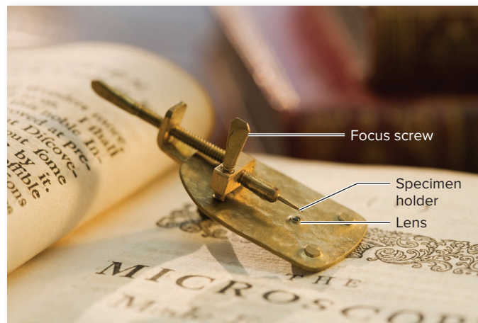
Figure 1.7 Leeuwenhoek’s microscope. A brass replica of a Leeuwenhoek microscope. The lens is held in front of one eye with the specimen holder facing outward.
