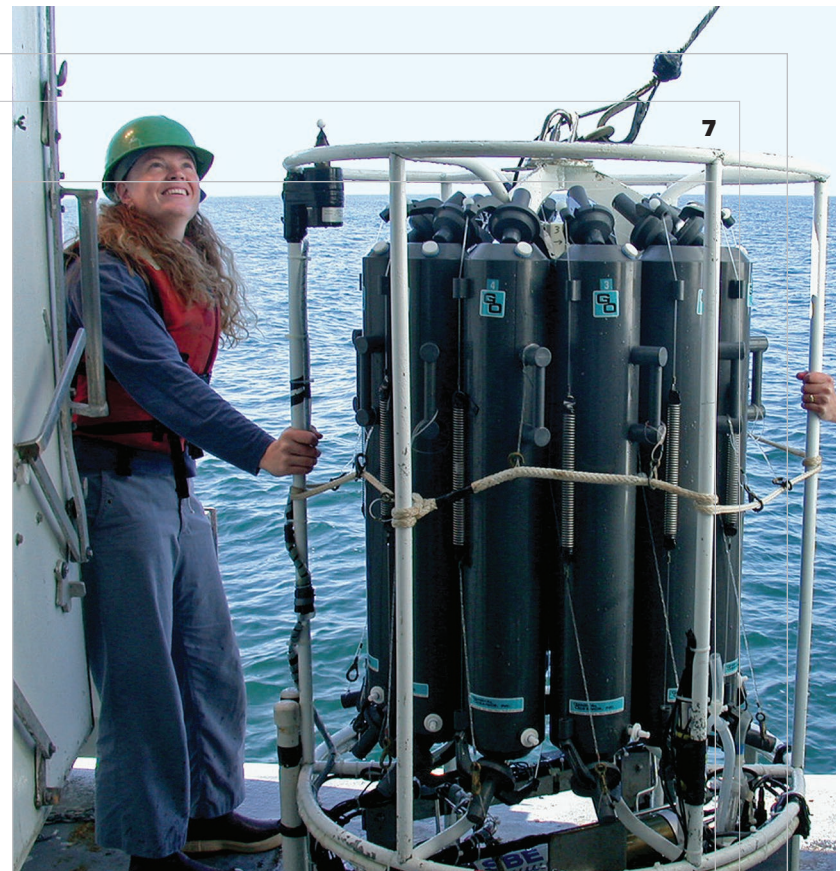
Figure 1.3 This instrument consists of numerous bottles that are submerged to collect water samples from the ocean. Source: National Oceanic and Atmospheric Administration
