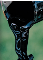
FIGURE 14.3 Synthetic crude oil is currently being produced from oil sand deposits (A) in Alberta, Canada. The hydrocarbons are in the form of bitumen, a highly viscous substance that is separated from the sand using steam. Photo (B) shows a bitumen sample whose viscosity has been lowered by heating. Approximately 45% of Canadian production involves strip mining (C); the remainder is produced by steam injection and pumping wells. (B) Syncrude Canada Ltd.; (C) Blackfox Images/Alamy Stock Photo.
