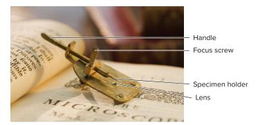
**FIGURE 1.1** Model of van Leeuwenhoek's Microscope The original made in 1673 could magnify an object almost 300 times. The object is brought into focus with the adjusting screws. Tetra Images/Alamy Stock Photo
