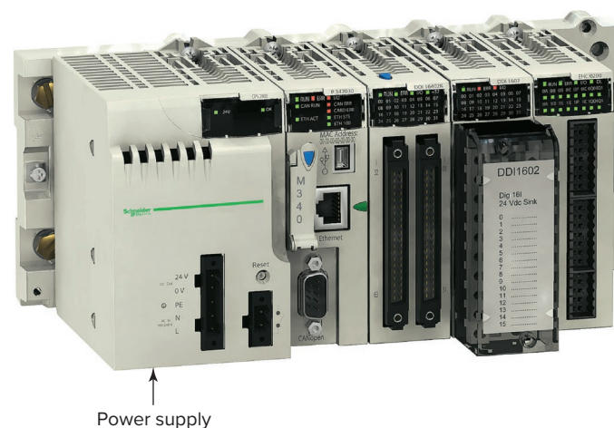
Figure 1-9 The power supply supplies DC power to other modules that plug into the rack.
