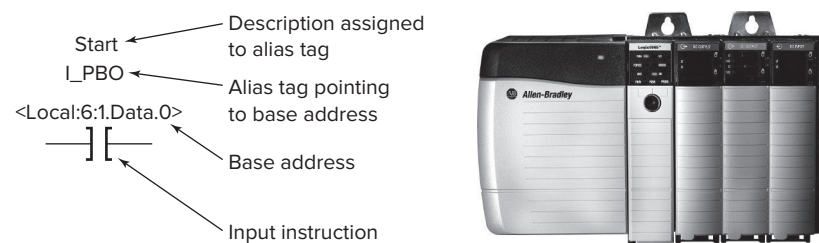
Figure 2-4 Allen-Bradley RSLogix 5000 tag-based addressing format. Source: Image Courtesy of Rockwell Automation, Inc.
