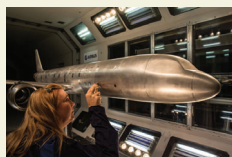
Figure 3 A model of an Airbus airplane is prepared for testing in a large wind tunnel.
