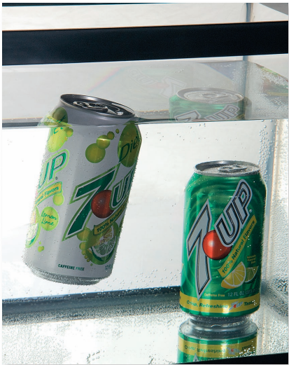
Although a can of a diet soft drink floats in water because it is less dense, a can of a regular soft drink that contains sugar is more dense than water so it sinks. Jill Braaten/McGraw Hill
