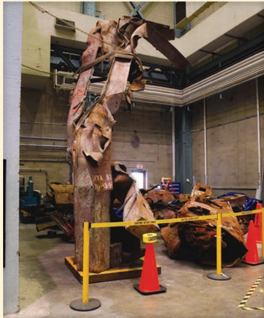
Figure 2-7 Steel from the World Trade Center under test at NIST.
