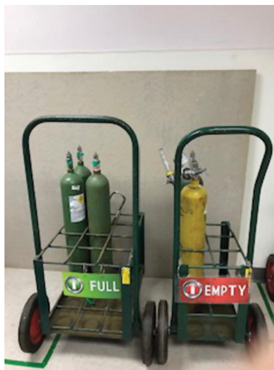
FIGURE 1-18 A. A portable cylinder cart allows for the cylinder to be safely stored for use during patient transport or ambulation. B. Multi-cylinder portable holders require labeling to reduce the potential of selecting an empty cylinder for patient use.
