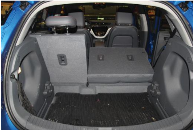
FIGURE 2-5 Rear seats in hatchbacks usually fold down to increase the luggage area.
