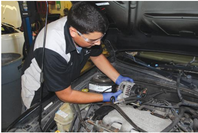
FIGURE 1-11 Light line technicians diagnose and replace the mechanical and electrical components of vehicles.
