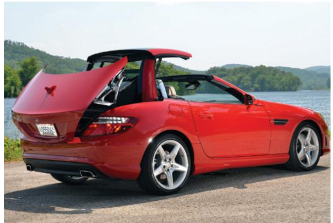
FIGURE 2-7 Hardtop convertibles have a hard roof that makes the vehicle look more like a conventional fixed-roof vehicle.
