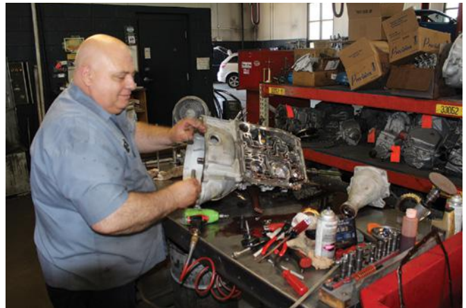
FIGURE 1-17 A transmission specialist rebuilding an automatic transmission.
