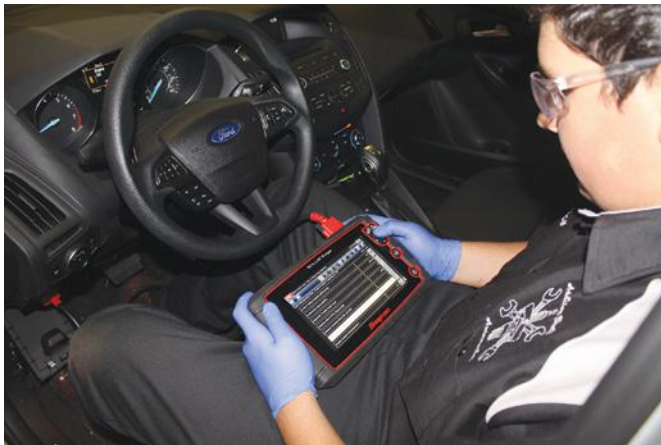
FIGURE 1-16 A drivability technician using a scan tool to diagnose a vehicle.
