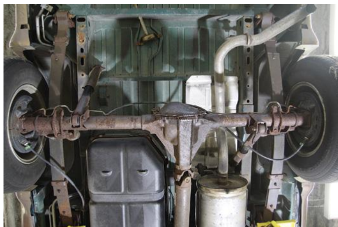
FIGURE 2-23 Rear axle assembly sending torque from the driveshaft to the rear wheels.
