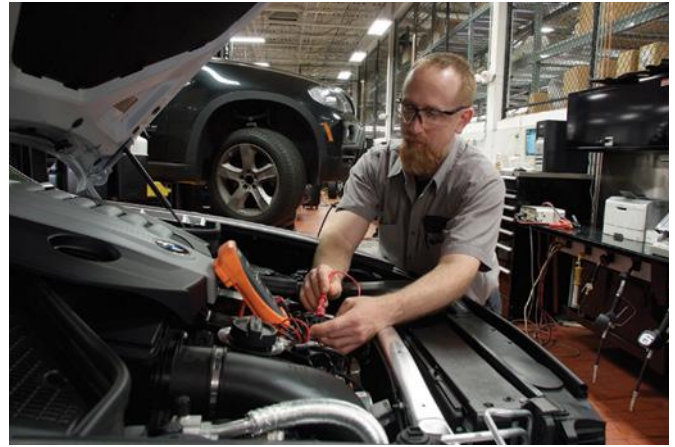
FIGURE 1-15 Electrical technicians install, maintain, identify faults with, and repair electrical wiring and computer-based equipment in vehicles.
