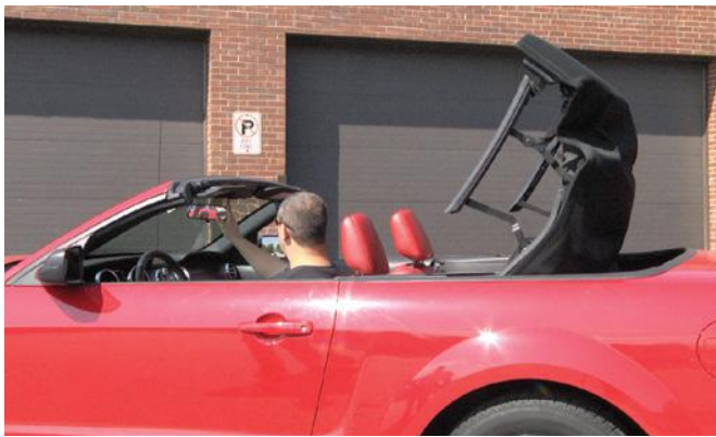
FIGURE 2-6 A convertible is an automobile that can convert from having an enclosed top to having an open top by means of a roof that can be removed, retracted, or folded away.
