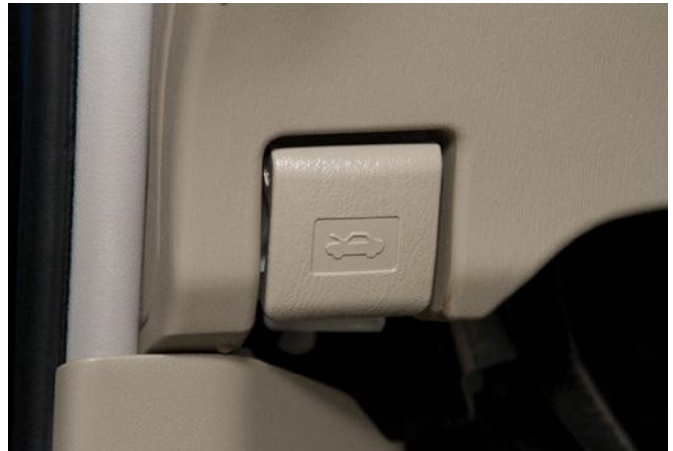
FIGURE 2-14 The engine compartment release may be located inside the passenger compartment under the dash, in the glove compartment, or on a doorjamb.
