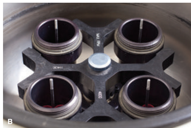
Figure 1.10 (A) Benchtop centrifuge. (B) Swinging-bucket rotor.
