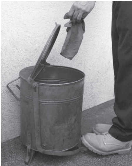
Figure 2-8 Place oily rags and other combustible waste in an approved container.
