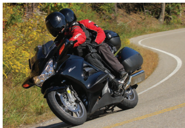
Figure 1-33 Sport-touring motorcycles are a combination sport bike and touring machine. They combine comfort with long-distance capabilities that allow two-up riding all day long while handling well at higher speeds when it is desired to do so.
