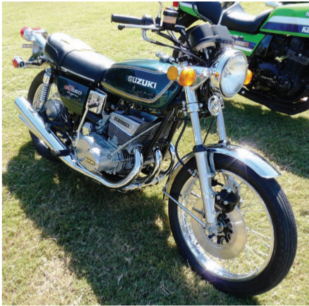
Figure 1-24 The Suzuki GT550 was a big hit in the United States when it was imported in the 1970s. The GT had a six-speed transmission and was very fast in its day and came in different engine displacements.
