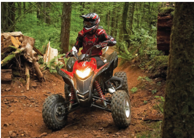
Figure 1-42 This example of a sport ATV is very popular and designed to be ridden on trails and on off-road race tracks. Note the distance between the wheels and fenders for suspension clearance.
