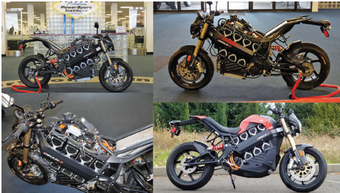
Figure 1-46 An all-electric powered motorcycle can be seen here with its bodywork off as well as on. As you can see, the machines look rather complex once all of its bodywork is removed. While they are complex, they are quite efficient.
