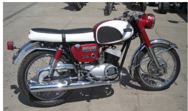
Figure 1-23 The Yamaha YM1 was a 305cc two-stroke that was produced from 1964 to 1966. It had an oil injection system to mix the oil with the gasoline and could reach speeds over 100 miles per hour.
