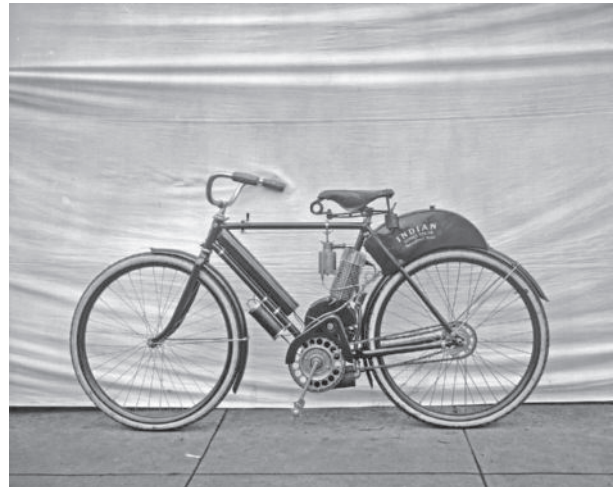
Figure 1-7 The first Indian motorcycle was produced in 1902 and was very similar in design to a bicycle.
