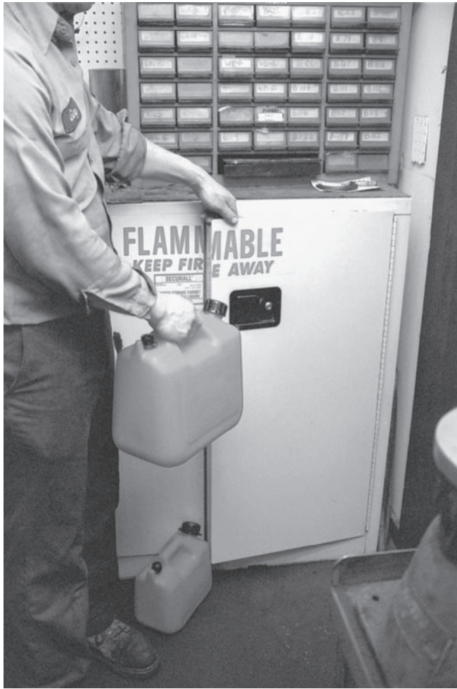
Figure 2-6 Always store flammable liquids in a cool, dry area away from ignition sources.
