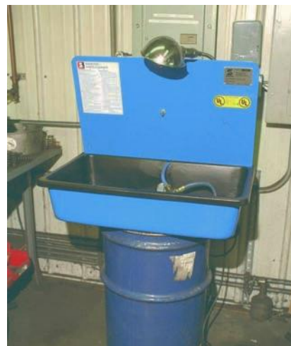
Figure 1-17 An aqueous parts-cleaning tank.
