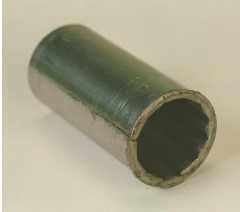
Figure 1-5 A worn-out impact socket must be replaced.
