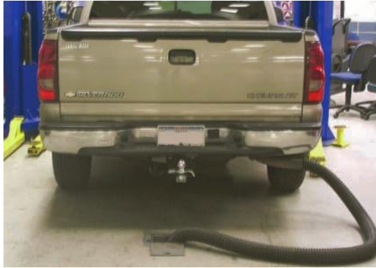
Figure 1-18 When running an engine in a shop, make sure the vehicle's exhaust is connected to the shop's exhaust ventilation system.
