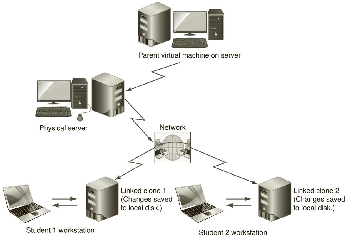
**Figure 1-13** Linking clones of virtual machines with VMware
