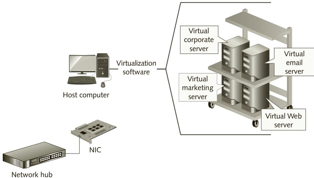
**Figure 1-4** Using virtualization to consolidate several servers onto a single host
