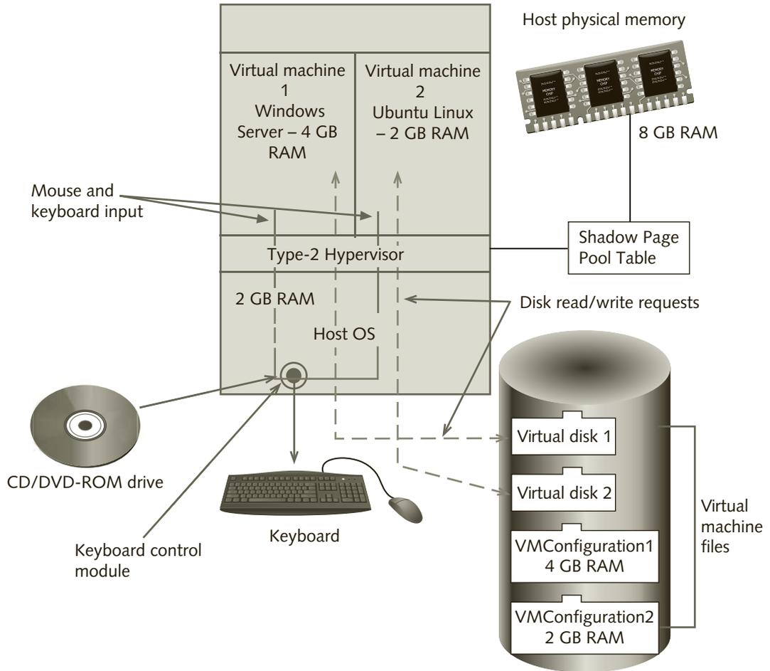
**Figure 1-2** Virtualization software operation
