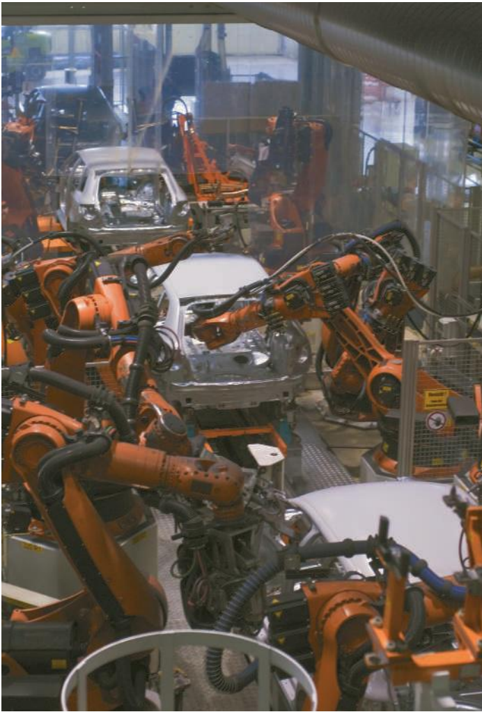
Figure 1-39 Automotive factories use industrial robots to weld car bodies.
