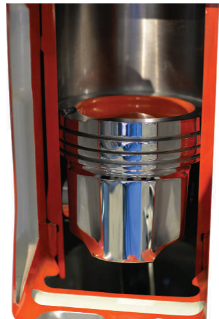
FIGURE 3-2 A Detroit Diesel DD5 piston shown with the cylinder cutaway: note the aggressive Mexican hat piston crown geometry used in this 5-liter engine.
