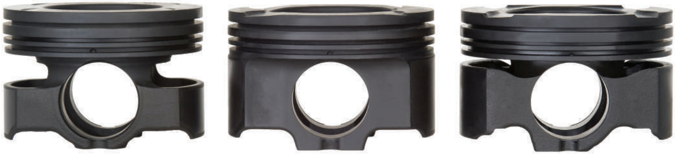
FIGURE 3-5 Examples of Mahle diesel engine pistons: the crown recesses in the image on the right are to accommodate cylinder head valve protrusion.
