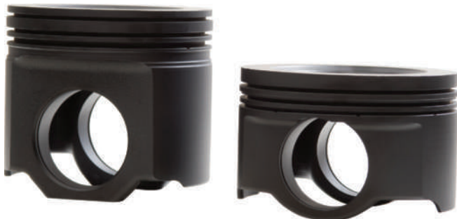
FIGURE 3–10 Two examples of three-ring configurations on trunk-type pistons.
