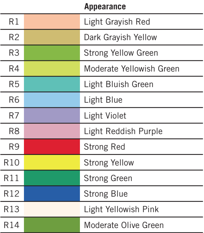
FIGURE 4.3 The CRI color chart reveals the light quality of a particular light source measured against natural light. It can be used to compare sources of the same type to determine better clarity.
