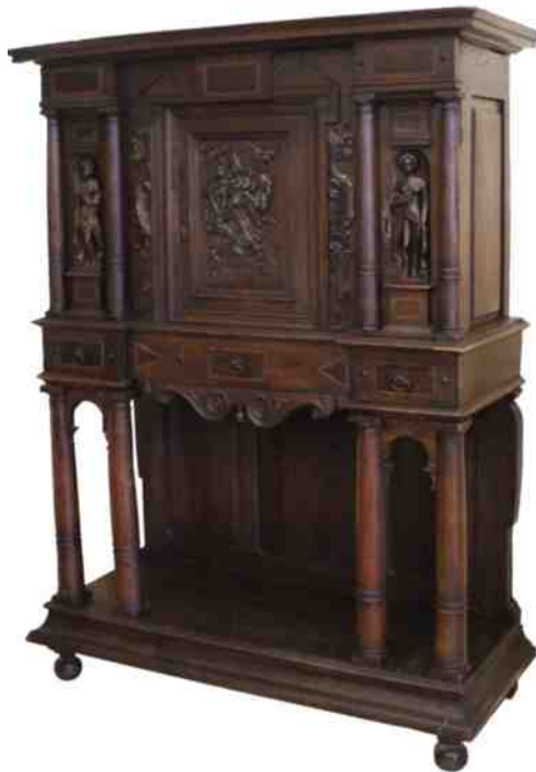
FIGURE 1.17 To create a turning, such as these legs, a sharp tool is held against the rotating piece of material.
