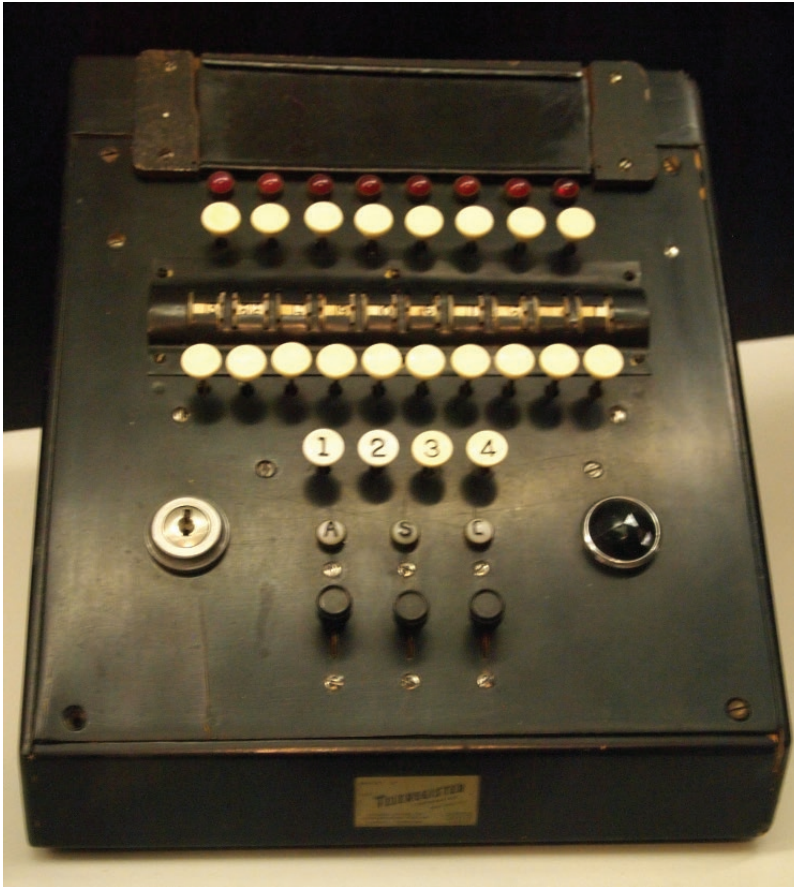
MagneTronic Reservisor – the first electronic reservations system, introduced in 1952 by American Airlines
