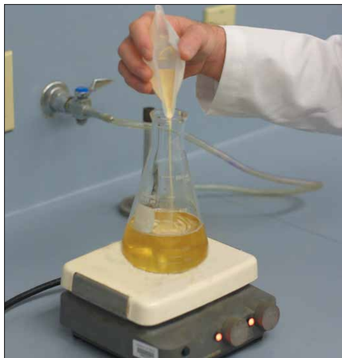
1.4 Mixing the Medium ■ The powder is added to a flask of distilled or deionized water on a hot plate. A magnetic stir bar mixes the medium as it is heated to dissolve the powder.
