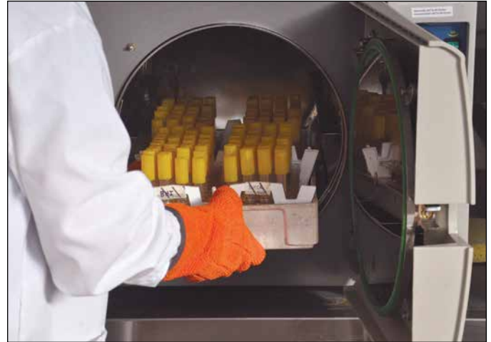
1.6 Autoclaving the Tubed Media ■ Media are sterilized in an autoclave for 15 minutes at 121°C. Shown are four racks of tubed media being removed from an autoclave. The tubes on the left are brain-heart infusion broth (BHI or BHIB) and they will be allowed to stand and cool. Once cool, they will remain liquid. The tubes on the right contain brain-heart infusion agar (BHIA), a solid medium, which is liquid when it is removed from the autoclave but will solidify as it cools due to the agar in it. The position of the tube as it cools will determine whether an agar deep tube or an agar slant is produced (Fig. 1.7). Note the angled sides of the racks that allow them to be tipped so the agar will solidify in a slant. Plated media are autoclaved in a flask and then dispensed into sterile Petri dishes (Fig. 1.8).
