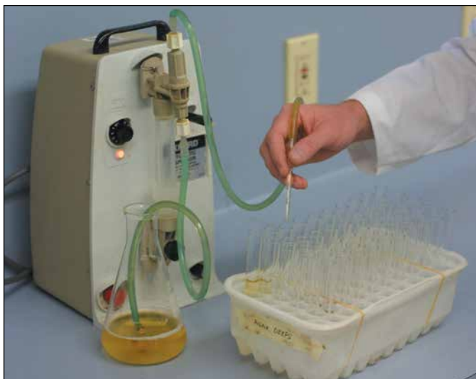
1.5 Dispensing the Medium into Tubes ■ An adjustable pump can be used to dispense the appropriate volume (usually 7 mL–10 mL) into tubes. Then, loosely cap the tubes.
