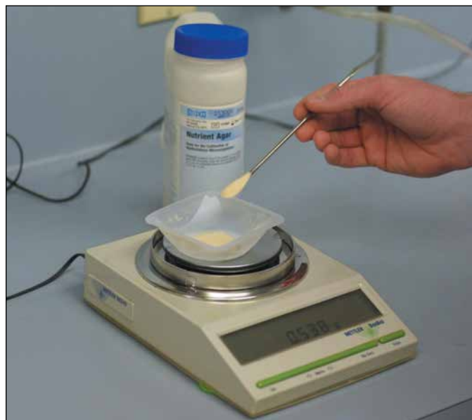
1.3 Weighing Medium Ingredients ■ Solid ingredients are weighed with an analytical balance. A spatula is used to transfer the powder to a tared weighing boat. Shown here is dehydrated nutrient agar, but the weighing process is the same for any powdered ingredient.
