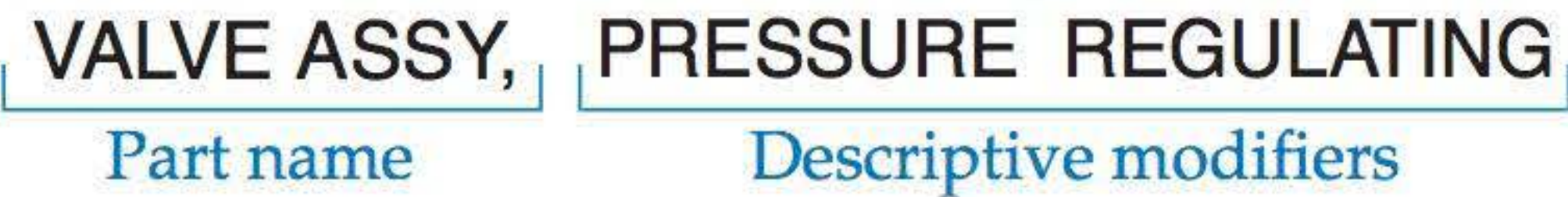
Figure 3-7. A part name often contains descriptive modifiers. When read out loud, the modifiers are read first and then the part name.
