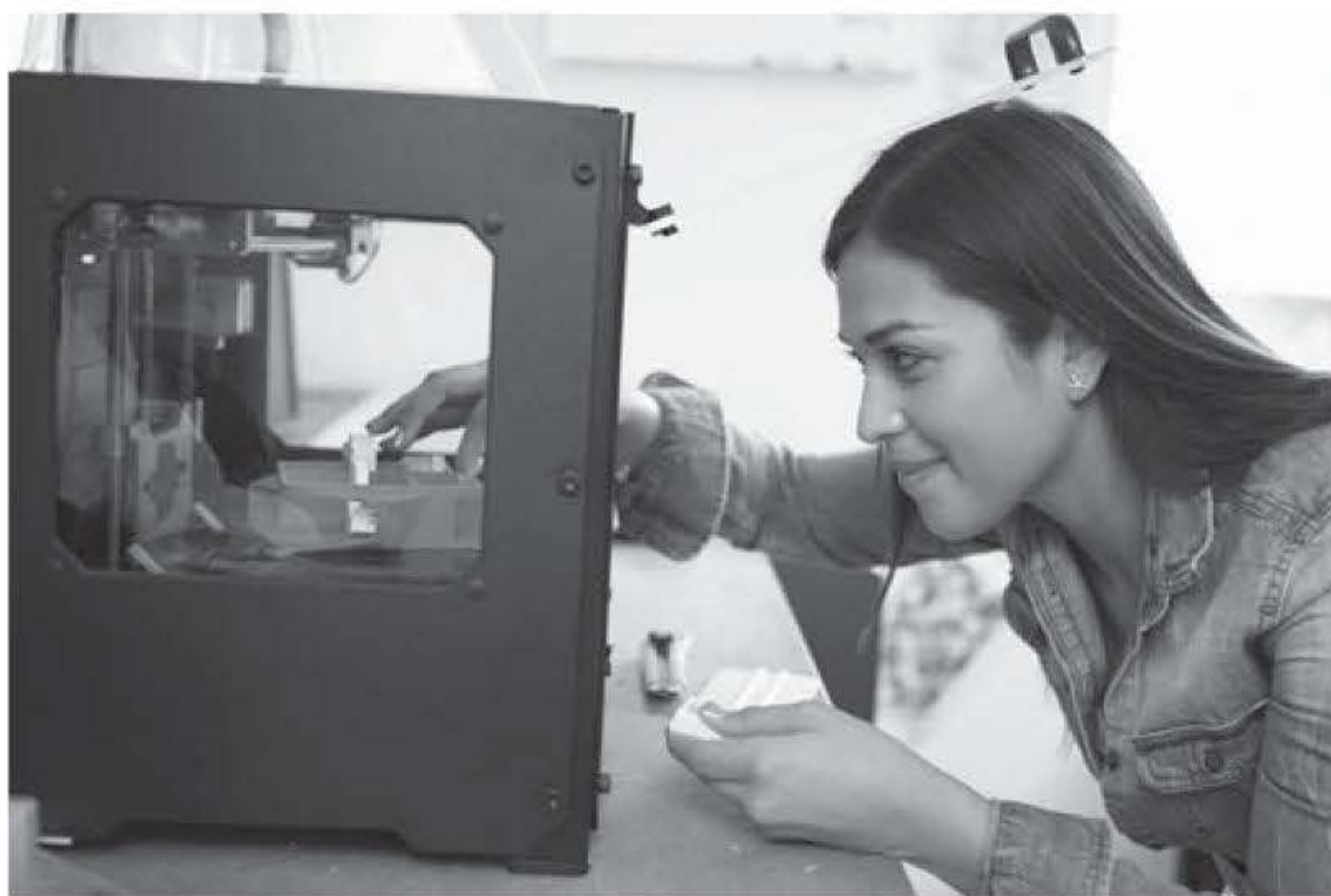
Figure 1-13. Desktop 3D printers can create plastic prototypes directly from a CAD file. The same technology can also create functioning parts for certain applications.
