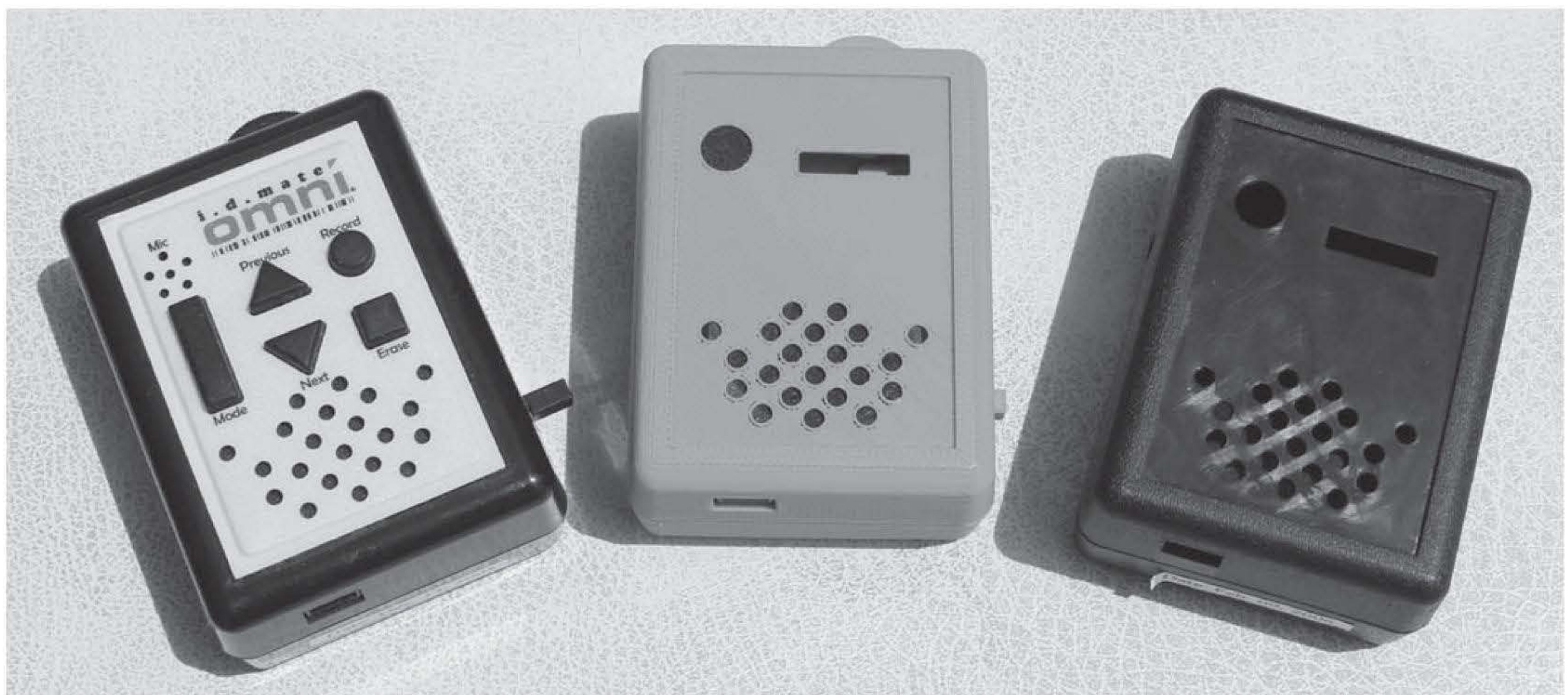
Figure 1-12. The original product on the left was redesigned and the plastic prototype in the center was generated directly from a CAD file. Although prints were not given to a modelmaker, drawings and sketches were useful in the design process. The prototype facilitated assembly, function, and comfort factor testing. The new molded plastic part is on the right.
